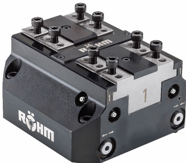
Image 2: In addition to a compact structure and a high degree of repetition accuracy, the KZS centric clamping vices deliver high clamping forces of up to 55 kN, an increased clamping range of 20% and a reduced interfering contour for an optimal chip flow (image: Röhms).
